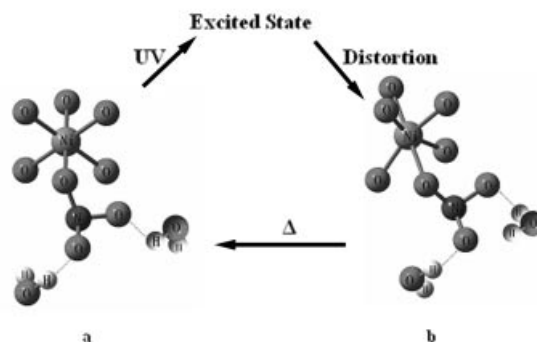
Figure 12. Photochromic mechanism in \text{NiAl-NO}_3\text{-LDH} : (a) structure before UV irradiation and (b) structure after UV irradiation.
